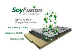
shingles, making them inflexible. SoyFusion Technology allows millions of microdroplets of oil to quickly penetrate the brittle protective top coating and saturate the weathering asphalt layer. This infusion rejuvenates the asphalt, restoring its flexibility and pliability. Roof Maxx also enhances adhesion of the protective mineral granules, which work like sunscreen, reflecting the sun's ultraviolet rays, the main source of physical/chemical degradation of roof materials.
