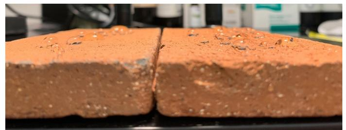
Bricks treated with Airable's formulation after exposure to accelerated weathering. The large, raised beads of water indicate a decrease in water surface tension.
