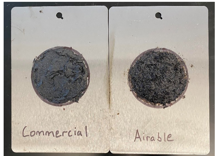
Side-by-side comparison of Airable's roof patch and a commercial product. The appearance and consistency are identical.
